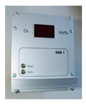
The gas analyser is provided with a chemical sensor.
